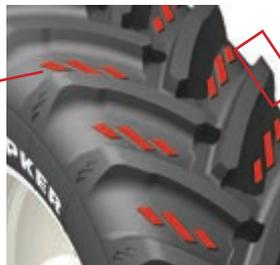
A lug pattern designed to protect the soil.
